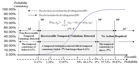
Fig. 2. Probability based temporal consistency model.
